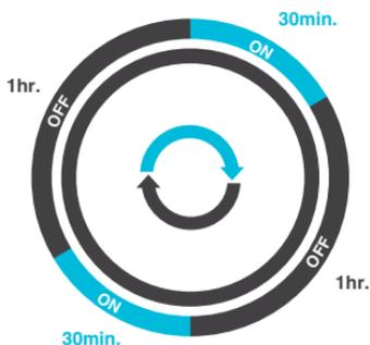
If there is a level set in OFF Mode other than zero, the devices will run at that level when triggered to turn off.
